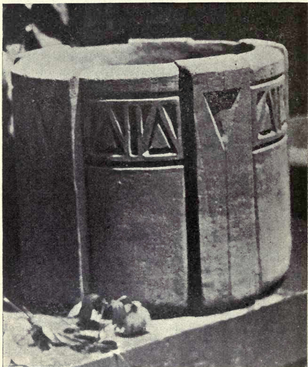
FIG. 64—SIMPLE FLOWER POT DESIGN IN CONCRETE, FROM PLASTER MOLD AND CLAY MODEL—PHILADELPHIA SCHOOL OF INDUSTRIAL ART
